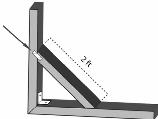
6. Attach the four  $90^\circ$  3" brackets (legs) at the four positions on the frame with  $\frac{1}{2}$ " screws.
